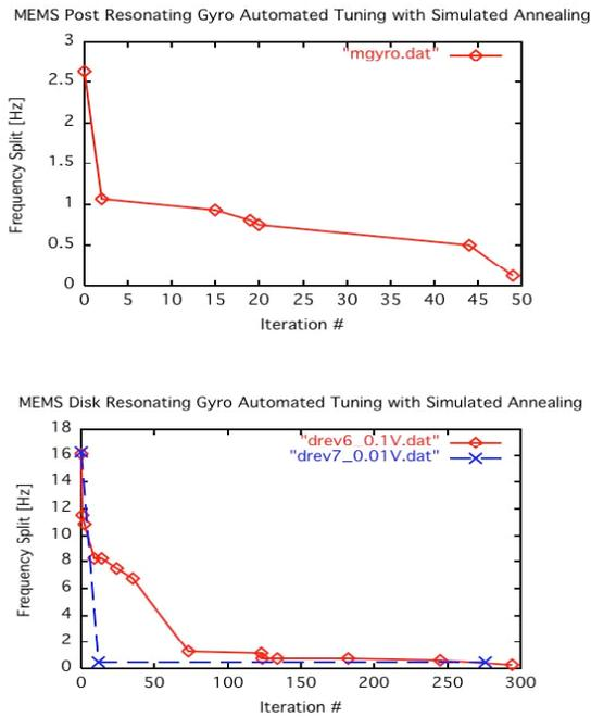
Figure 5. Frequency split as a function of Simulated Annealing Iterations: (top) for the MEMS post-resonator gyroscope; (bottom) for the MEMS disk-resonating gyroscope.
