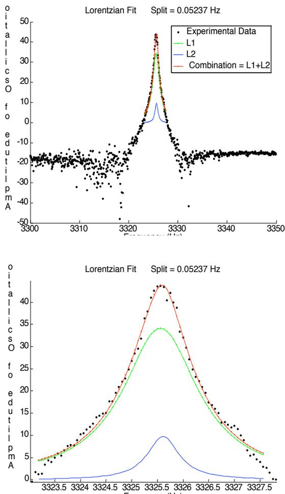
**Figure 8. Frequency response (top: 50Hz band, bottom: 5Hz band) after tuning using the modified genetic algorithm. The Y axis is measured in dB. The tuning frequency split is 52mHz. The optimized values of the four bias voltages are: B1 = 4.00V BT1 = 4.00V B2 = 14.00V BT2 = -16.00V. The bottom picture shows a zoom of the frequency split over a 4Hz band.**
