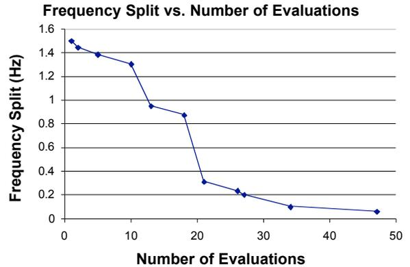
Figure 6. Frequency split as a function of number of evaluations used by the Dynamic Hill Climbing algorithm.
