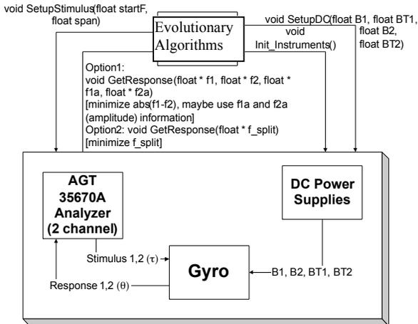
**Figure 2. Software interface between the Simulated Annealing/Modified Genetic Algorithm and the Instrumentation Platform using a GPIB programmable power supply DC voltage and a signal analyzer. The Simulated Annealing and GA/Hill Climbing are running on a PC, which controls the bias voltages and receives the frequencies of both resonance modes.**
