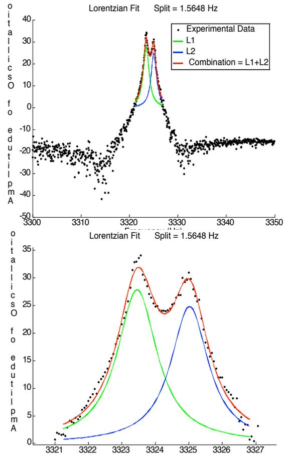
**Figure 7. Frequency response (top: 50Hz band, bottom: 6Hz band) before tuning using the modified genetic algorithm. The frequency split is 1555mHz. The Y axis is measured in dB. The initial values of the four bias voltages are: B1 = 14.00V BT1 = 14.00V B2 = 14.00V BT2 = 14.00V. The bottom picture shows a zoom of the frequency split over a 6Hz band.**
