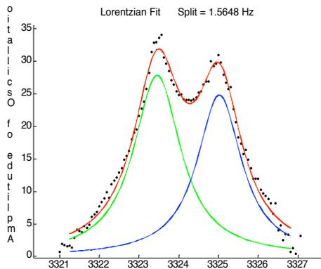
**Figure 4. Fitting the sum of two Lorentzian functions to the frequency response experimental data. The green and blue curves are Lorentzian functions and the red curve is the sum of the two functions. The experimental data points are plotted in black.**
