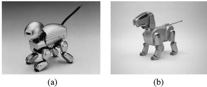
Fig. 1. Sony’s entertainment robots: (a) OPEN-R prototype; (b) ERS-110.
