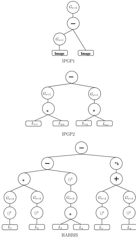
**Figure 3: Tree representation for three different interest point detectors. From top to bottom: IPGP1, IPGP2 and Harris. It can be easily observed the simple structure found by the GP search when compared with the most popular interest point detector of computer vision.**
