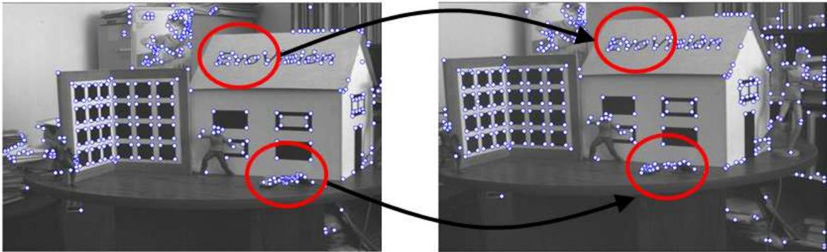
**Figure 1:** A stereo pair taken at the EvoVisión Laboratory, notice how interest points can be used to compute the correspondence between both images. The interest points depicted on both images were obtained with the IPGP2 presented in this work that outperforms past human designs.
