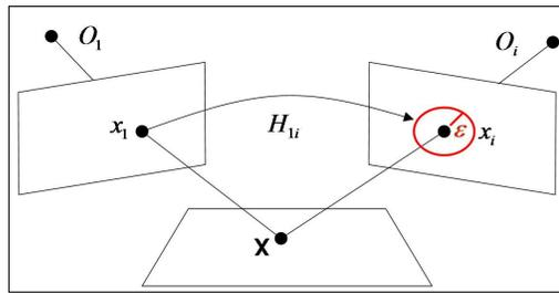
**Figure 2: A 3D point  $X$  is projected onto points  $x_1$  and  $x_i$  on images  $I_1$  and  $I_i$  respectively. Point  $x_1$  is said to be repeated by  $x_i$ , if a point is detected within a neighborhood of  $x_i$  of size  $\epsilon$ . For planar scenes  $x_1$  and  $x_i$  are related by the homography  $H_{1,i}$ .**
