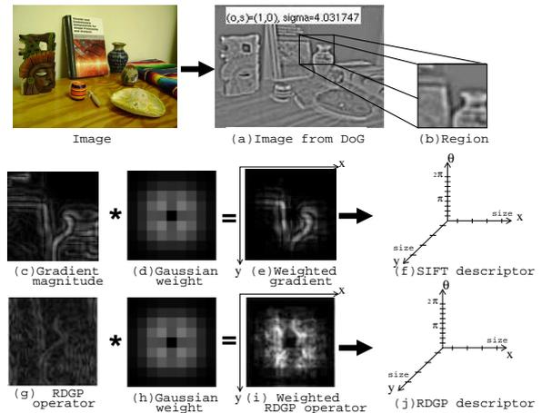
Figure 2: Local image descriptor operator used within SIFT: c) gradient magnitude g) RDGP.
