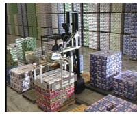
Fig. 6. Order assembly using the temporary stacks of the picking area.
