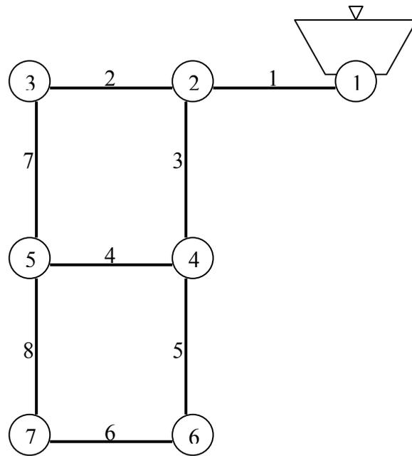
Figure 4. Two-loop water distribution network.
