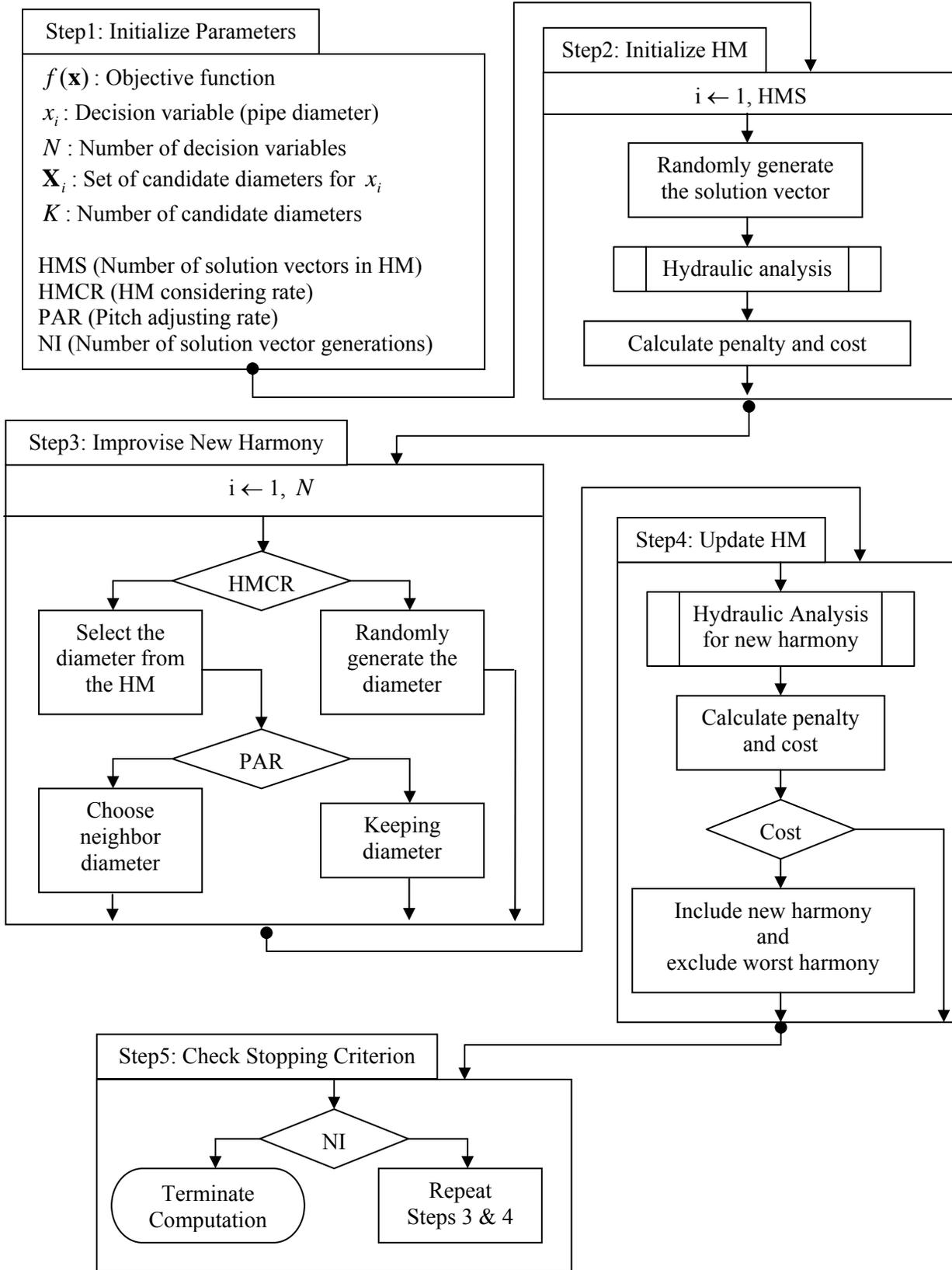
Figure 1. HS procedure for water distribution network design.
