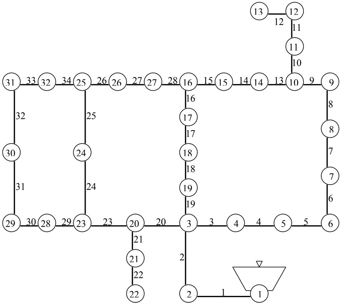
Figure 5. Hanoi water distribution network.
