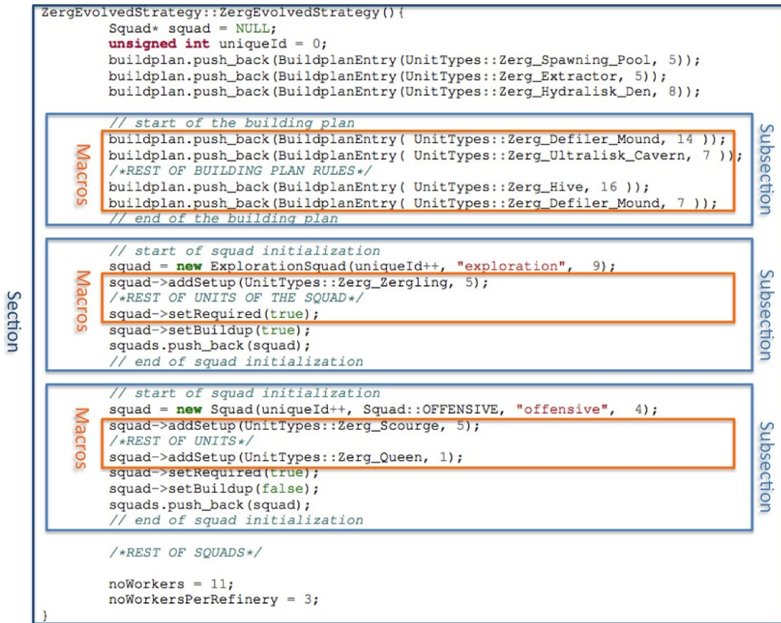
Fig. 3. Example of a generated initialization method.
