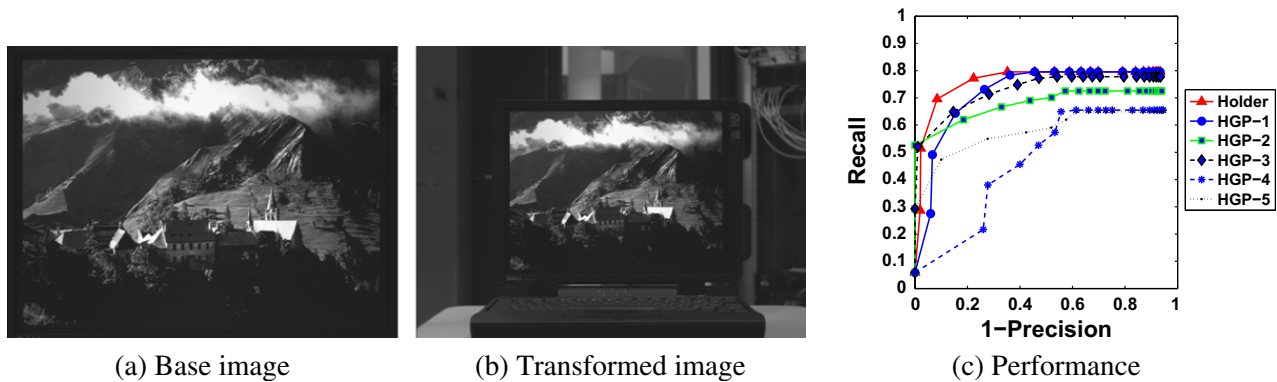
Fig. 19. Recall/1-Precision curves for the Laptop image pair. The transformation between (a) and (b) is a scale change or zoom.
