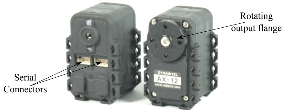
Figure 6.1: Back and front views of the Dynamixel AX-12+ motor. Each motor’s rotating output flange is attached to a robot leg. A quadruped robot therefore has four such motors and a hexapod has six, which are connected in a daisy chain using serial connectors. One end of the daisy chain is plugged into a CM-2+ microcontroller board (Figure 6.2) running an evolved neural network controller. This setup allows the neural network to communicate with all four motors and thus control the leg movements of the robot. Reprinted with permission from Robotis (2010); annotations added.
