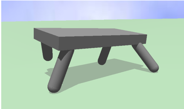
Figure 4.1: The quadruped robot model. The legs are attached to the body by hinge joints with axes of rotation tilted sideways, allowing the legs to make full circular rotation. Locomotion is achieved by coordinating the circular movements of the legs. This model is a simple but physically realistic platform that also allows scaling up to more complex robots by adding more legs or by increasing the legs' degrees of freedom.
