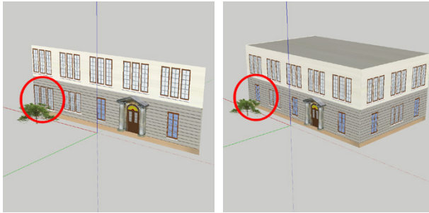
(a) Auto-generated front face by the proposed method in SketchUp (b) Manually completed building model
